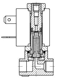
It can be **normally open** (3/2 NO). In this case when the coil isn't energised the inlet orifice is open to the user port. Exhaust port is closed. When connected to an electrical supply, the inlet orifice closes, at the same time the exhaust port is opened and connected with the user port.
