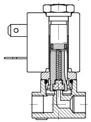
It can be **normally open** (2/2 NO). In this case the orifice is open, the inlet feeds through the outlet. When connected to an electrical supply the orifice is closed. The operation, in both cases depends only on the magnetic field produced by the coil. These solenoid valves are able to work at **zero pressure**.
