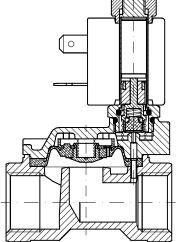
They are available with an **assisted lift** design pilot operated by diaphragm and **normally closed** (2/2 NC). In these models the plunger is mechanically attached to the diaphragm and controls the central pilot orifice and the stroke of the main seal.
