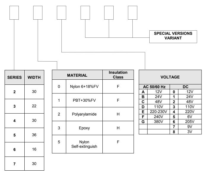
Example : 30B Coil width 22 mm in Nylon 6+18% Fibre Glass Insulation class F Voltage 24V 50/60Hz power 8VA
