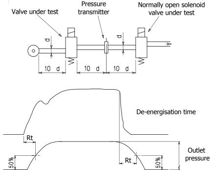
The response time depends from the type of valve, the nature of the medium, the pressure and the current (AC or DC), if these value are measured at the moment of electrical connection or disconnection.
